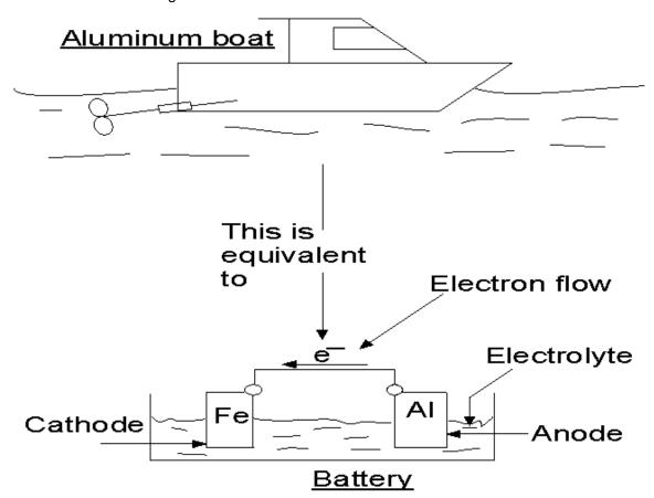
For galvanic corrosion to occur, there must be an electrical circuit. This means there must be a path for the electrons to travel between the two dissimilar metals and there must be a path through the electrolyte for the ions to travel. Additionally, the chemical reaction at the cathode usually requires the presence of oxygen in the electrolyte.
